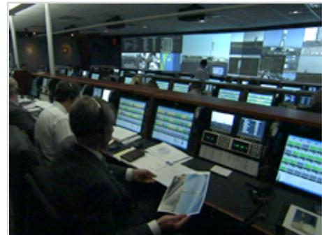
From their consoles in the Mission Director's Center at Cape Canaveral Air Force Station, launch controllers monitor a launch vehicle and spacecraft prior to liftoff. The Telemetry and Communications Group provides data, voice, video and telemetry for NASA launches around the globe -- even as far away as Alaska and the Marshall Islands. Image credit: NASA
